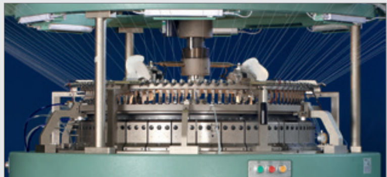
knitting head (3-feeder cam boxes)
