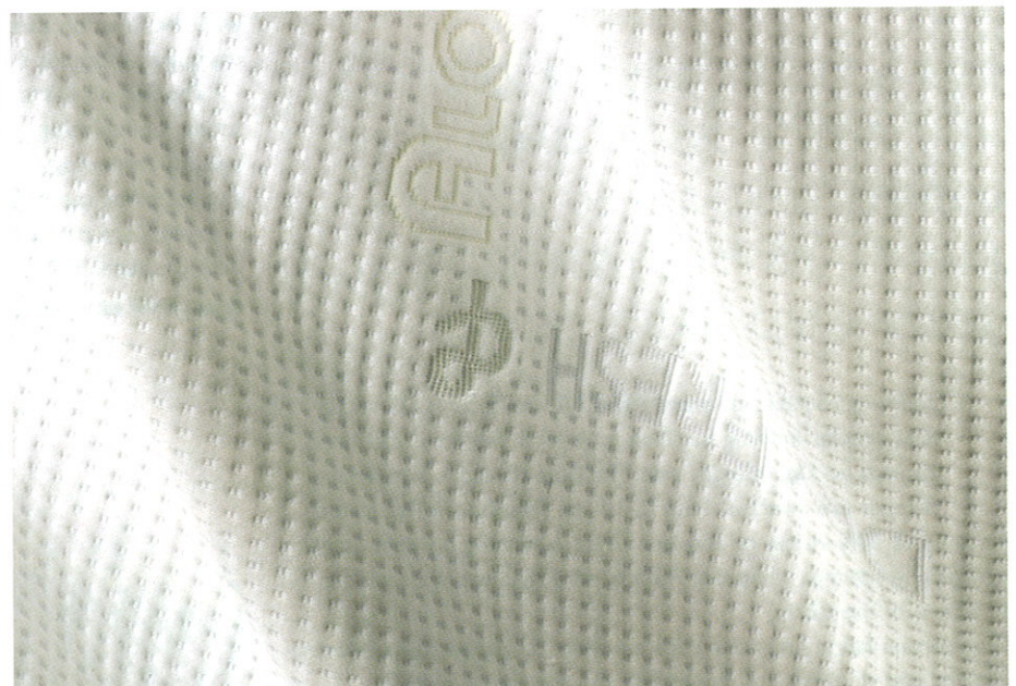
Samples of mattress ticking fabric produced on Terrot's UCC572M series.
