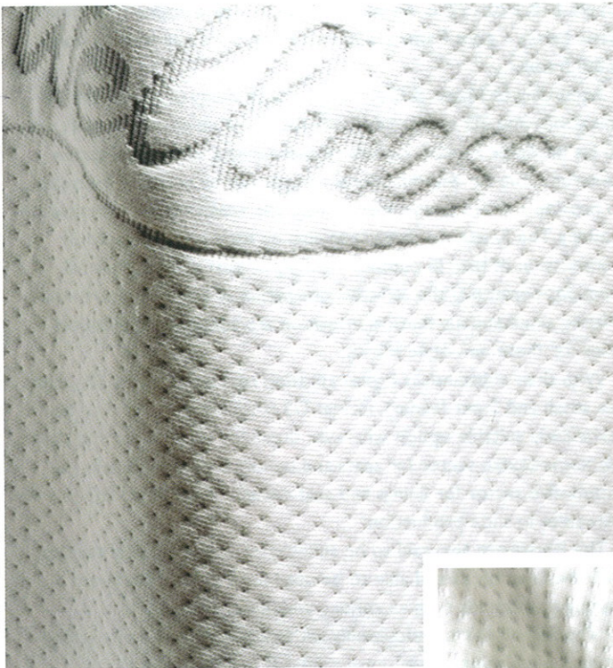
Samples of mattress ticking fabric produced on Terrot's UCC572M series.
