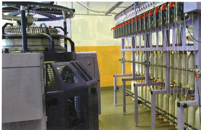
F132-AJ spin-knit machine (Terrot)
