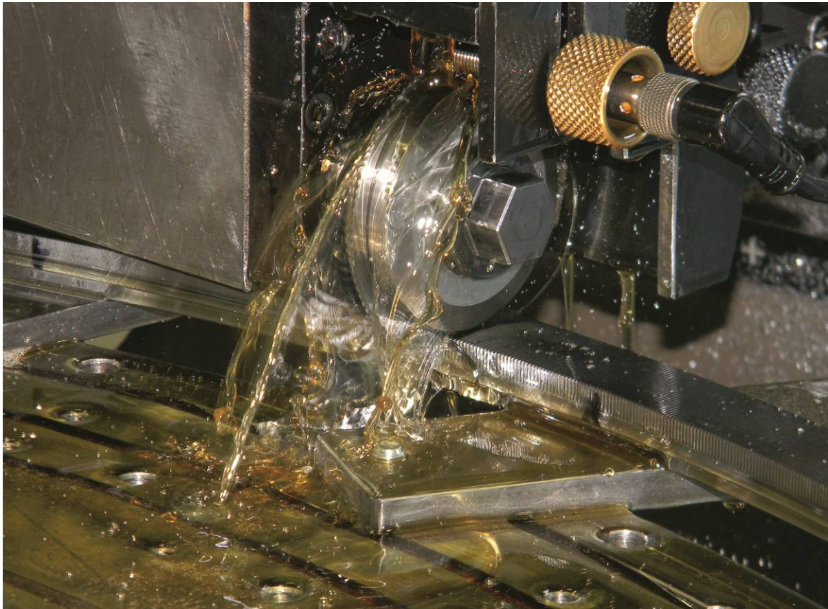
Photo 2: Detailed view of sinker ring cutting
