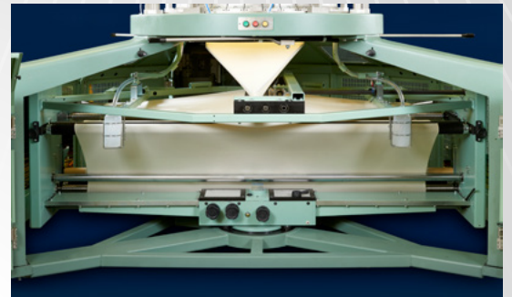
OW3/1 frame with open width take-down
